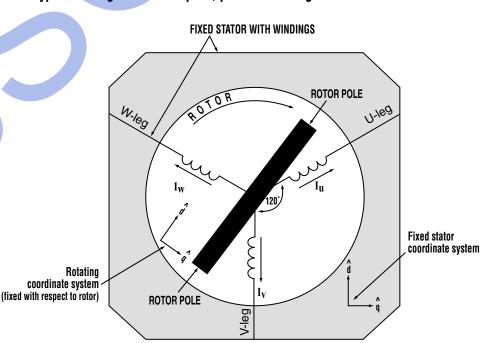
NOTE: Current polarities  $l_U$ ,  $l_V$ , and  $l_W$  are defined such that the resulting magnetic fields have the directions shown. In other words, positive u-leg current will produce a magnetic field vector oriented as shown by the arrow labeled  $l_U$ .
